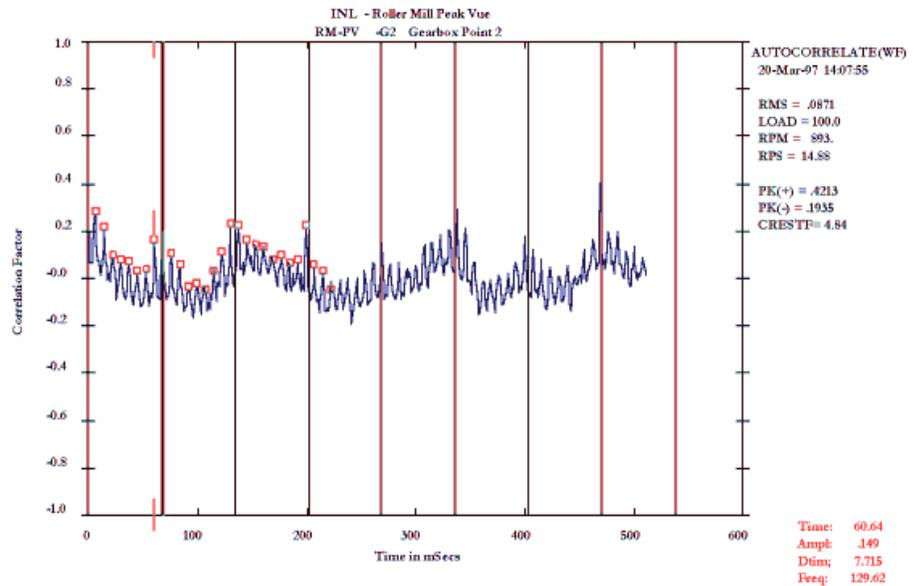
The autocorrelation coefficient function computed from the PeakVue time waveform in Fig. 7 is presented in Fig. 8. The inner race defect is clearly evident with amplitude modulation at running speed. The peak g levels for an inner race are generally not as large as for those accompanying an outer race defect. This is expected since the stress waves accompanying an inner race defect will experience attenuation in reaching the outer
