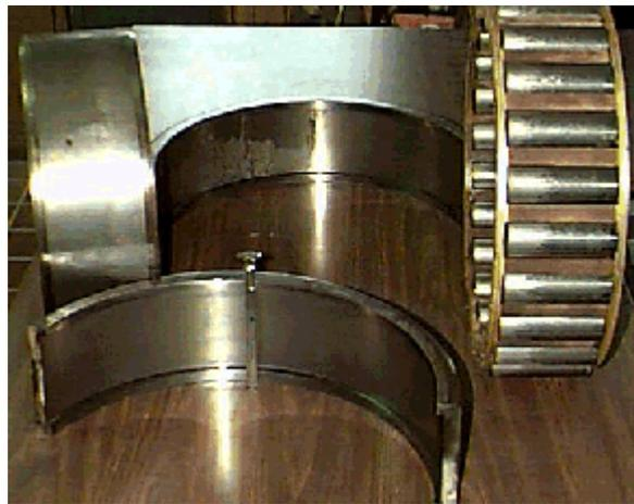
The impacting levels trended from 18 g's in July to a high of 37 g's in September. The levels had decreased to 14 g's in October prior to a bearing replacement.
