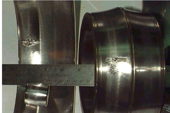
In this case, normal vibration data did identify the fault; however, the low levels observed did not place the fault at a level of significant concern. The impacting levels identified in PeakVue, excess of 30 g's, raised the concern level and initiated planning for replacement.
