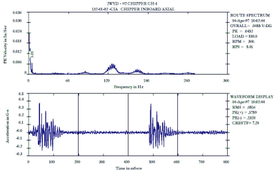
Figure 12. PeakVue Spectra and time waveform from inboard axial on chipper.
