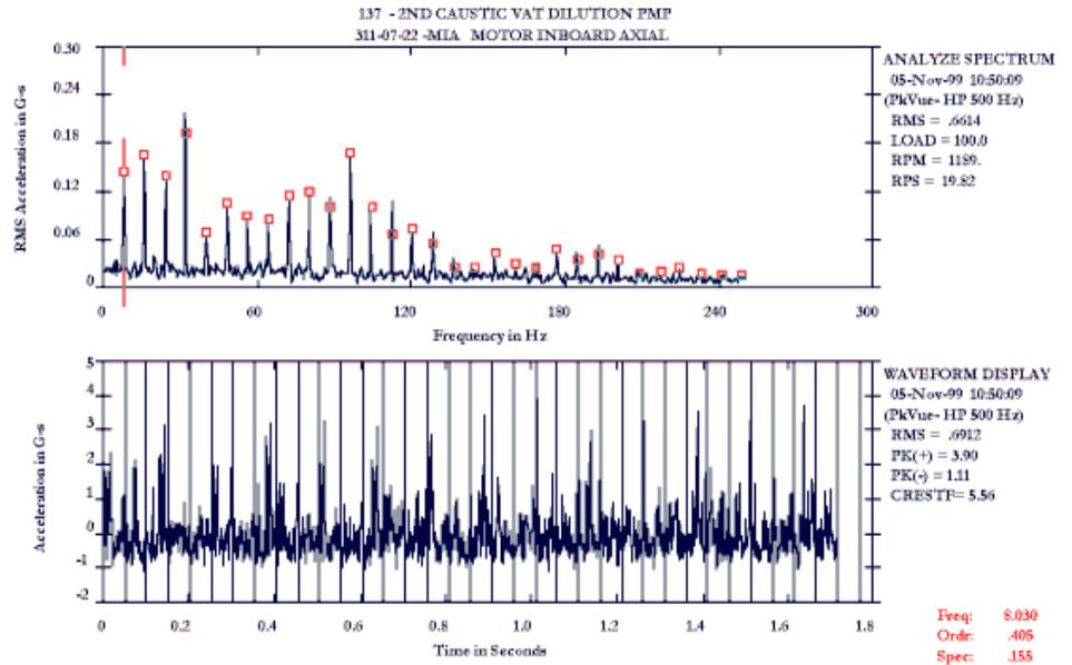
The impacting levels are 5 g's which are not excessive for this speed machine but definitely indicative of a problem. The spectral data is dominated with cage and many harmonics. This is a NSK NU 318 bearing which has 13 rolling elements.
