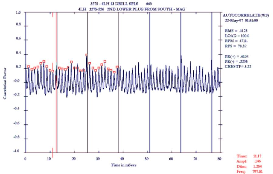
The PeakVue spectra and time waveform for a spindle with a confirmed inner race defect are presented in Fig. 9. The inner race defect at 797.86 (10.2 orders) Hz is identified with side banding (twice running speed is dominant). The autocorrelation coefficient function computed from the PeakVue time waveform is presented in Fig. 10. The dominant activity here is at the inner race defect frequency. The bearing was replaced. The bearing had deep spalling on the inner race
