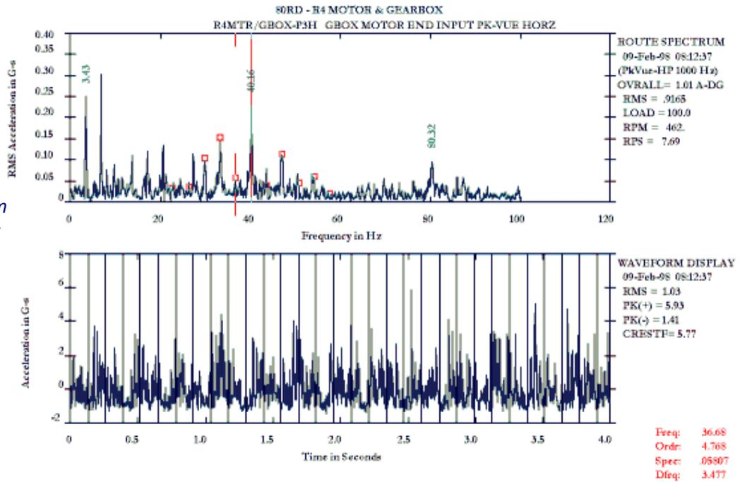
The bearing was replaced and PeakVue data acquired on February 12, 1997. The impacting level had decreased to less than 1 g. The normal vibration never showed any indication of a bearing problem.
